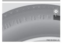
In addition to the load bearing index, load index ① may be imprinted after the letters that identify speed index ⑥(▷ page 330) on the sidewall of the tire.
