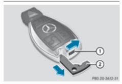
▶ Push release catch ① in the direction of the arrow and at the same time remove mechanical key ② from the SmartKey. For further information about:
