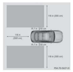
Blind Spot Assist monitors the area up to 10 ft (3.0 m) behind your vehicle and directly next to your vehicle, as shown in the diagram. For
