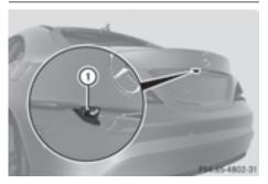
Rear view camera ① is in the trunk lid handle. The rear view camera is an optical parking and maneuvering aid. It uses guide lines to show the area behind your vehicle in the Audio/COMAND display.
