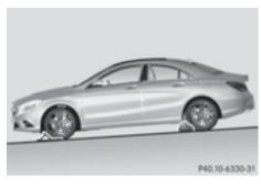
Securing the vehicle on slight downhill gradients
