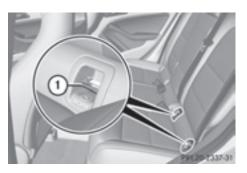
▶ Install the LATCH-type (ISOFIX) child restraint system on both LATCH-type (ISO-FIX) securing rings (1). Comply with the child restraint system manufacturer's instructions when installing the LATCHtype (ISOFIX) child restraint system.
