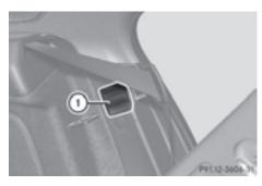
▶ Insert the seat belt into seat-belt extender (1).
