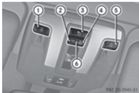
Front overhead control panel
