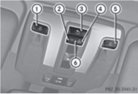
Front overhead control panel
