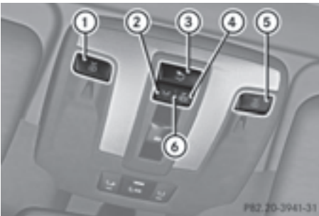
Front overhead control panel
