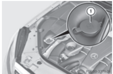
Example: adding fluid to the windshield washer system
