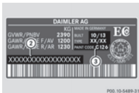
Example: vehicle identification plate (Canada only)
