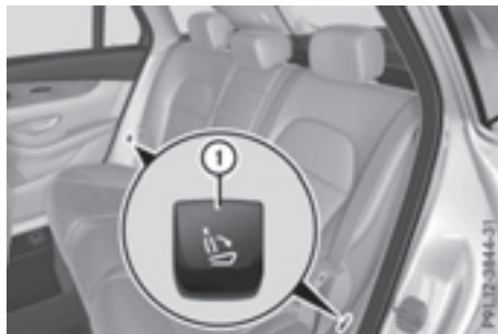
Release handle next to the seat backrest (vehicles with EASY-PACK tailgate only)
