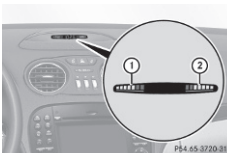
Front area warning indicators
