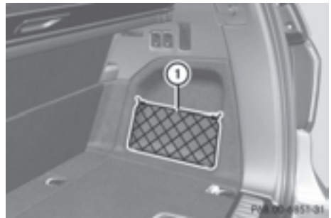
① Stowage net in cargo compartment Observe the loading guidelines (▷ page 340) and the safety notes regarding stowage spaces (▷ page 341).
