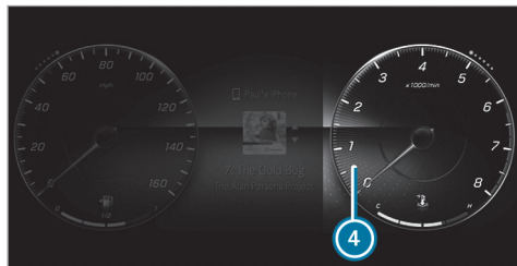
④ Display content, right (example: tachometer)
