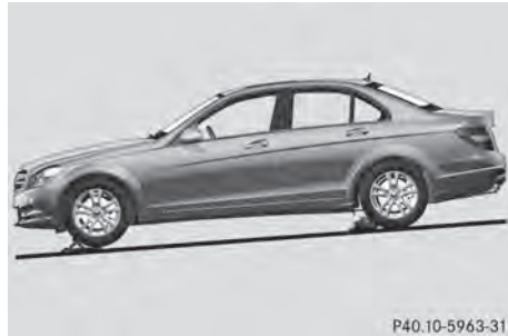
Securing the vehicle on slight downhill gradients
