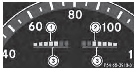
Warning display for the front area
