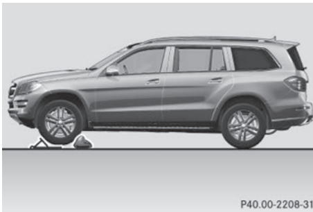
Securing the vehicle on level ground
