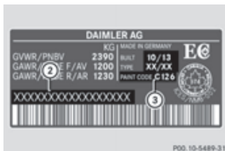
Example: vehicle identification plate (Canada only)
