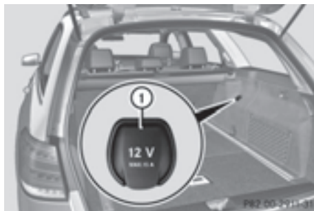
Power socket in the cargo compartment (Wagon)
