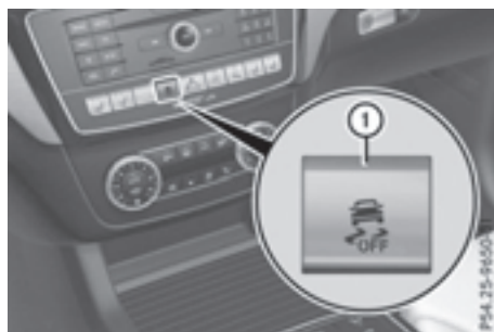
ESP® OFF button (except Mercedes-AMG vehicles)
