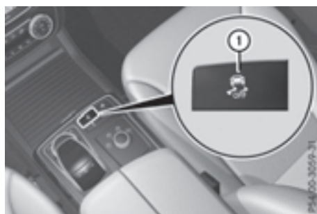
ESP® OFF button (Mercedes-AMG vehicles)
