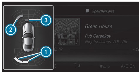
Parking Assist PARKTRONIC warning display (vehicles without front and rear view camera)
