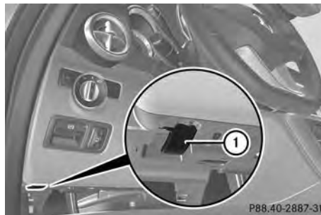
Hood release lever in driver's footwell
