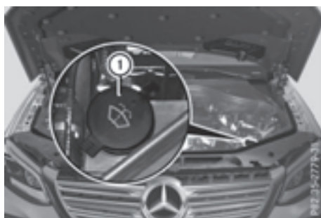
Example: washer fluid reservoir
