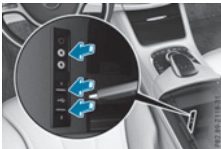
Connections in the storage compartment under the armrest in vehicles without rear climate control
