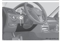
Driver's knee bag ① deploys under the steering column. It is deployed together with the front air bags. The driver's knee bag is designed to operate together with the front air bags in frontal impacts if certain thresholds are exceeded. The driver's knee bag operates best in conjunction with correctly positioned and fastened seat belts.
