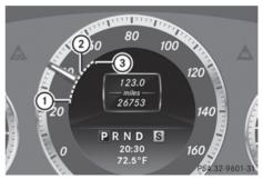
When DISTRONIC PLUS is activated, one or two segments (2) in the set speed range light
