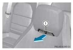
You can adjust the blower output of AIRSCARF vents (1) using the AIRSCARF button ( $\triangleright$  page 112).
