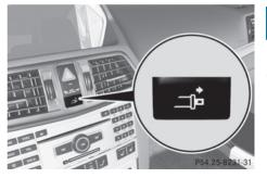
You can also extend seat-belt extender (1) by using the seat-belt extender button in the center console.
