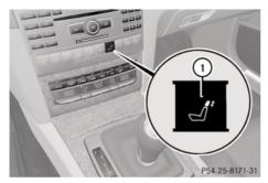
Press rear seat head restraints button ①. The rear seat head restraints and AIRCAP wind screen rise upwards.
