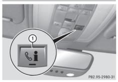
Press MB Info call button ①. This initiates a call to the Mercedes-Benz Customer Assistance Center. The indicator lamp in MB Info call button ① flashes while the connection is being made. The Connecting Call message appears on the multifunction display. The audio system is muted.
