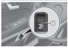
► **To open:** pull remote operating switch for trunk lid ① until the trunk lid opens.
