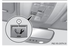
Press Roadside Assistance button ①. This initiates a call to the Mercedes-Benz Customer Assistance Center. The indicator lamp in Roadside Assistance button ① flashes while the call is active. The Connecting Call message appears on the multifunction display. The audio output is muted.
