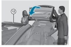
► Lift the soft top out of the soft-top compartment and guide it forwards in the direction of the arrow onto windshield frame <sup>(1)</sup>/<sub>2</sub>.
