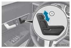
To adjust the head restraint height: slide switch for head restraint adjustment (1) up or down in the direction of the arrow.
