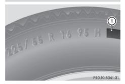
In addition to the load bearing index, load index (1) may be imprinted after the letters that identify speed index (6) on the sidewall of the tire ( $\triangleright$  page 338).
