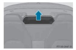
Pull the AIRCAP wind screen out of the guide rails in the direction of the arrow.
