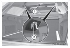
▶ Pull the cargo net up by tab (1) and hook it into eyelets (2).
