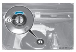
► Turn DEF cap ① counter-clockwise and remove it.
