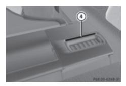
▶ Make sure that red lock status indicator (4) is no longer visible. The combined cargo cover and net will otherwise not be locked in place.
