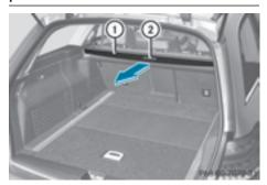
➤ To extend: pull cargo compartment cover ① back by grab handle ② and clip it into the retainers on the left and right.
