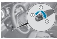
You can set the specified minimum distance for DISTRONIC PLUS by varying the time span between one and two seconds. With this function, you can set the minimum distance that DISTRONIC PLUS keeps to the vehicle in front, dependent on vehicle speed. You can see this distance in the multifunction display (> page 195).
