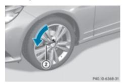
► Using lug wrench ②, loosen the bolts on the wheel you wish to change by about one full turn. Do not unscrew the bolts completely.
