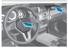
Driver's air bag (1) deploys in front of the steering wheel; front-passenger front air bag (2) deploys in front of and above the glove hox.
