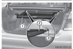
➤ To install: insert retainer ② of box ① into slots ③
