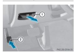
If you brake the vehicle with the parking brake, the brake lamps will not light up.
