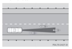
DISTRONIC PLUS has not yet detected the vehicle in front on the edge of the road,
