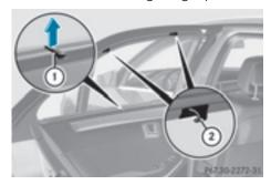
▶ To extend: pull the roller sunblind out by tab (1) and hook it onto retainers (2) at the top of the window.
