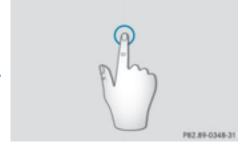
Use one finger to press the touch-sensitive surface until you reach the pressure point. A menu, an option or an application is started.
