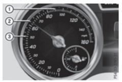
Example: DISTRONIC PLUS displays in the speed-ometer
