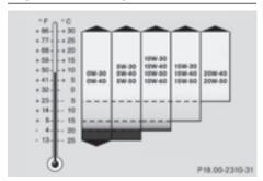
Viscosity describes the flow characteristics of a fluid. If an engine oil has a high viscosity, this
