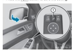
If you have switched the Auto. Mirror Folding on and you fold the exterior mirrors in using button 1, they will not fold out automatically ( $\triangleright$  page 105).
