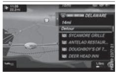
Highway information enables the use of the traffic jam function. The remaining route on the highway in this case is blocked in the direction of travel from the selected exit.
