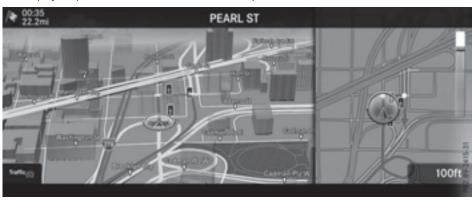
The change of direction is performed when the light-colored bar on the right drops down to 0 ft and the current vehicle position symbol has reached the white change-of-direction point.
