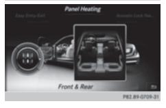
The panel heating function warms the surfaces with which the vehicle occupants frequently come into contact. Activation of the panel heating via the multimedia system as described below only works if seat heating is activated (see the vehicle Operator's Manual).
