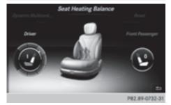
The balance function controls the distribution of heat on the seat backrest and cushion.
