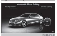
When the Automatic Mirror Folding function is activated, the outside mirrors fold in automatically as soon as you lock the vehicle from the outside. The outside mirrors fold out automatically again as soon as you unlock the vehicle.
