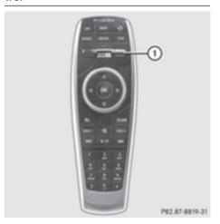
You can use the remote control to operate one of the two rear screens at a time. To do so, you must switch the remote control to the desired screen.
