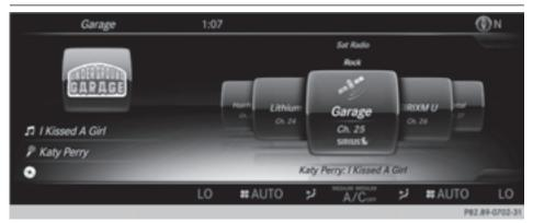
The additional display area occupies the left-hand or right-hand third of the display. The additional display area allows you to view various items of additional information. For instance, you can display an album cover in media mode or a permanent display, such as a small navigation map, in the additional display area.
