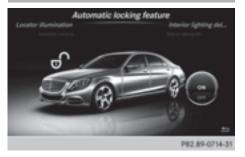
When the automatic locking feature is switched on, the vehicle is locked automatically when the ignition is switched on and the vehicle is traveling faster than walking pace.
