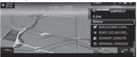
Highway information facilitates route guidance to a POI (e.g. rest stops, highway exits) and use of the traffic jam function. The remaining route on the highway in this case is blocked in the direction of travel from the selected exit.
