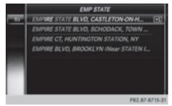
► To select an address: press the controller. The search results are displayed. Exact hits are shown at the very top of the list. Hits are listed alphabetically. The search term is highlighted in orange for exact matches.
