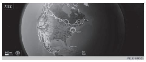
The navigation map and satellite images are shown in globe projection. This allows for a realistic map display free from distortion in all map scales.
