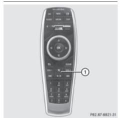
► Press button ① on the remote control. The sound is switched on/off.
