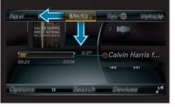
Back button Press and hold: Switches to the basic menu
