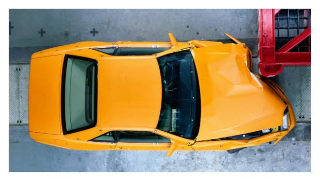
vehicle, so that more of the car's mass and structure can help to dissipate the forces before they reach the cabin. Perhaps no automaker has more experience in this realworld approach, with the structural design of the newest Mercedes—Benz models reflecting literally generations of further development, refinement and enhancement of this revolutionary concept.
