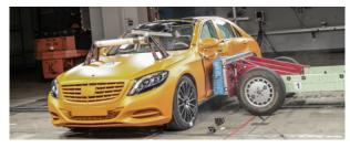
As with frontal impacts, the rigid passenger compartment is a prerequisite for effective occupant protection. In a side impact, the deformation zone available for protection of the occupants is very small in comparison to a frontal impact and requires special measures, including a very rigid side wall structure, cross-cabin reinforcements, as well as a highly effective side-impact restraint system.
