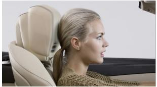
The crash-responsive NECK-PRO<sup>®</sup> active head restraints for the driver and front passenger are standard equipment in many Mercedes-Benz models. This important safety feature improves the protection of the front occupants during a rear impact by reducing the risk that the occupant will experience whiplash injury.
