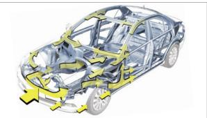
Mercedes-Benz body structures are systematically engineered to manage the forces of a variety of collision types. The basis for the high level of safety provided by a Mercedes-Benz is the fundamental principle of passive safety developed by Béla Barényi—consisting of a highly
