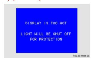
If the message "DISPLAY IS TOO HOT ..." appears, the display is too hot. For protection the light will be shut off. When the display has cooled down the light will be automatically switched on.
