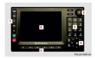
Using the MCS (Modular Control System) operating unit it is possible to operate the radio, tape deck, single CD player, CD changer, telephone and navigation systems and to adjust the system settings.
