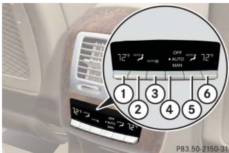
Automatic climate control panel, rear
