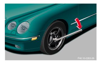
11. Lower vehicle. Remove jack and insert jack tube cover.
