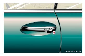
6 Infrared receiver in driver's door handle
