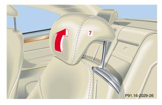
Adjust the head restraint angle (7) by hand. Push or pull the head restraint in direction of arrow.
