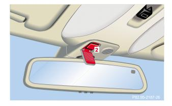
Press the SOS button (2) briefly (for longer than 2 seconds). The indicator lamp in the SOS button (2) will flash until the emergency call is concluded. Wait for a voice connection to the Response Center.
