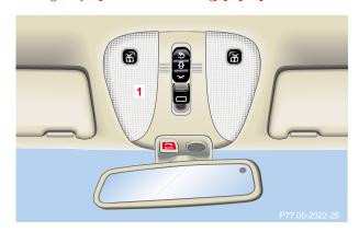
The sliding/pop-up roof can be opened or closed manually should an electrical malfunction occur.
