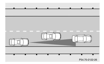
The Distronic system's detection zone is relatively narrow at the start and becomes broader as it senses further from the vehicle. Thus, Distronic may not recognize another vehicle coming into your path close to the front of your vehicle. You must be prepared to intercede with braking or steering as necessary. A vehicle not traveling directly in front of you could cause detection problems, the actual distance to that vehicle really being much shorter.
