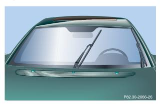
To prevent damage to the hood or the wipers, the wiper arms should only be folded forward in the position shown above.
