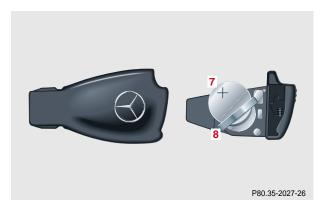
Change batteries (7), inserting new ones under contact spring (8) with plus (+) side facing up.
