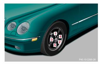
12. Using the wrench, tighten the five bolts evenly, following the sequence illustrated, until all bolts are tight.
