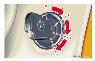
O The electronic key can be withdrawn in this position only. The electronic key can be removed only with the selector lever in position "P". After removing the electronic key or with the electronic key in starter switch position 0 or 1 the selector lever is locked in position "P".
