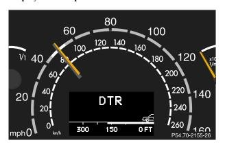
When Distronic system is activated, one or two segments around the speed stored in memory light up in the speedometer dial.
