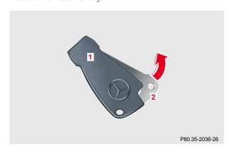
The electronic reserve key is without remote control functions, plus removable mechanical key.
