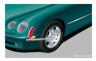
4. Remove the two-piece wheel wrench from the vehicle tool kit and assemble. Using the wrench, loosen but do not yet remove the wheel bolts.
