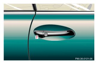
7 Infrared receiver in passenger door handle
