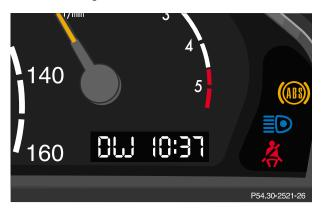
The current selector lever position is indicated in the gear range indicator display. The automatic gear shifting process can be adapted to specific operating conditions using the selector lever.
