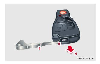
Insert mechanical key (4) in side opening (5) to open latch. Press briefly (do not use mechanical key as lever) to release battery compartment.
