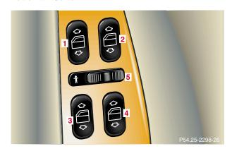
The control panel is located on the driver's door. Switches for:
