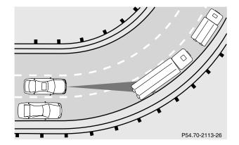
Traveling through turns or bends in the roadway may result in Distronic detecting a moving vehicle traveling in front but not in your lane of travel, causing your vehicle to brake late or unexpectedly. You must be prepared to intercede with accelerator or brake application as necessary.
