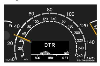
With the electronic key in starter switch position 2, the distance warning lamp l in the speedometer dial comes on and goes out with the engine running.
