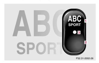
The switch is located on the center console Press the switch when the engine is running:
