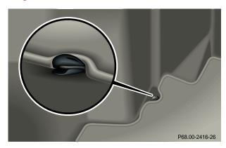
Inside the trunk are six cargo tie-down hooks. Secure cargo by applying even load on the hooks using a cargo net.
