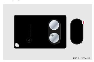
Pry open cover (1) (e.g. by using a narrow blade screw driver) and remove batteries.
