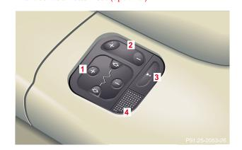
The switch clusters are located on the sides of the front seats.
