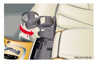
To close: Fold second cup holder in direction of arrow (3) until it engages.
