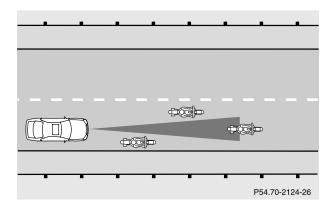
A narrow vehicle (e.g. a motorcycle) is only recognized when entering the area scanned by Distronic. You must apply the service brakes to gain sufficient distance to the vehicle ahead.
