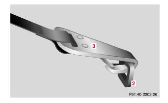
To secure a tether strap to the anchorage, securely fasten the hook (3), which is part of the tether strap, to the anchorage ring (2). For safety, please make sure that the hook has attached to the ring beyond the safety catch, as illustrated.
