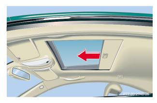
With the roof closed or tilted open, a screen can be slid into the roof opening to guard against sun rays. When sliding the roof open, the screen will also retract.
