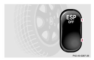
ESP control switch located on center console.
