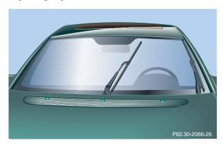
To prevent damage to the hood or the wipers, the wiper arms should only be folded forward while in the position shown above.
