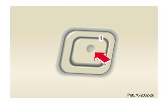
Coat hooks (1) are located on the headliner above the rear windows.
