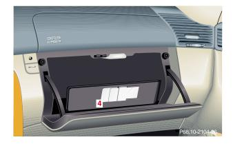
4 The glove box lid is equipped with a container (4) for coins and small accessories.
