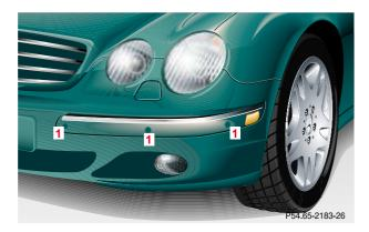
1 Sensors located in bumpers (front bumper shown) A total of 10 sensors (1) monitor the vehicle's front and rear areas. Six sensors are located in the front bumper, four sensors in the rear bumper.
