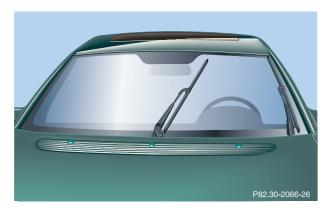
To prevent damage to the hood or the wipers, the wiper arms should only be folded forward in the position shown above.
