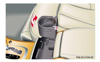
Press button (2) to open the second cup holder. The cup holder opens automatically.
