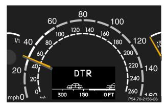
With the electronic key in starter switch position 2, the distance warning lamp l in the speedometer dial comes on and goes out with the engine running.
