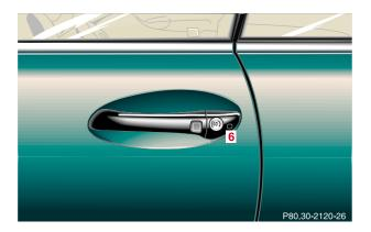
6 Infrared receiver in driver's door handle
