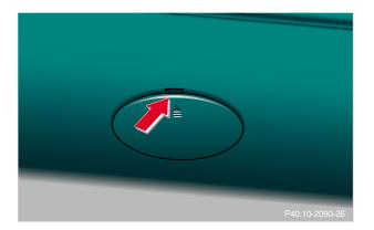
5. Remove the protective cover from the jack support tube opening by inserting the screwdriver (supplied in the tool kit) in the opening and prying it out.
