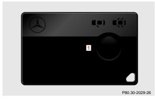
The KEYLESS-GO-card (1) does not have a removable mechanical key.
