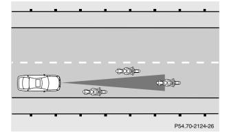
A vehicle changing lanes at close range is only recognized when entering the area scanned by Distronic. You must apply the service brakes to gain sufficient distance to the vehicle ahead. A narrow vehicle (e.g. a motorcycle) is only recognized when entering the area scanned by Distronic. You must apply the service brakes to gain sufficient distance to the vehicle ahead.
