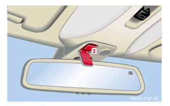
Press the SOS button (2) briefly (for longer than 2 seconds). The indicator lamp in the SOS button (2) will flash until the emergency call is concluded. Wait for a voice connection to the Response Center.
