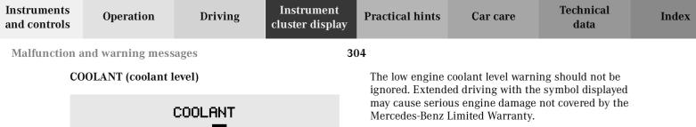
In cases of major or frequent minor coolant loss, have the cooling system checked at your authorized Mercedes-Benz Center as soon as possible.
