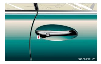
7 Infrared receiver in passenger door handle
