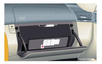
4 The glove box lid is equipped with a container (4) for coins and small accessories.
