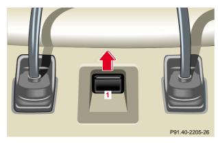
This vehicle is provided with tether anchorages for a top tether strap at each of the rear seating positions.
