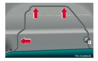
The maintenance-free battery is located in the trunk under the right-hand wheel well cover panel.
