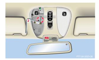
Obtain crank (2) (supplied with vehicle) and insert through hole.
