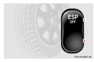
ESP control switch located on center console.
