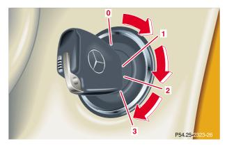
**0** The electronic key can be withdrawn in this position only. The electronic key can be removed only with the selector lever in position "P". After removing the electronic key or with the electronic key in starter switch position 0 or 1 the selector lever is locked in position "P".
