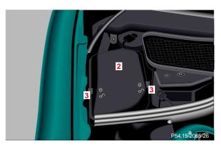
2 Fuse box in engine compartment, right-hand side
