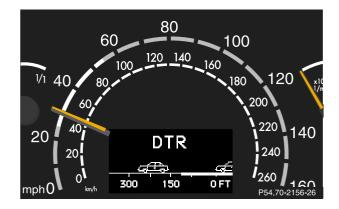
If a vehicle is detected ahead, those segments in the speedometer dial light up that indicate the speed range from the speed of the vehicle in front up to the Distronic stored speed.
