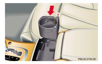
Press button (4) to unlock cup holder and fold into the storage compartment until it engages. Close the storage compartment.
