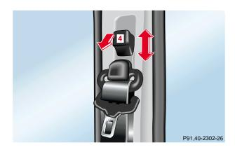
4 Button for belt outlet height adjustment
