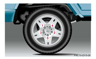
With the vehicle lowered to ground, tighten the five bolts evenly using the wrench. When tightening follow the sequence illustrated, until all bolts are tight. Observe a tightening torque of 97 ft.lb. (130 Nm).
