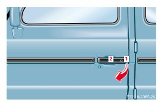
To open the door, press the lock cylinder (1) and pull on the door handle (2).
