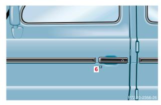
6 Infrared receiver at the driver's door
