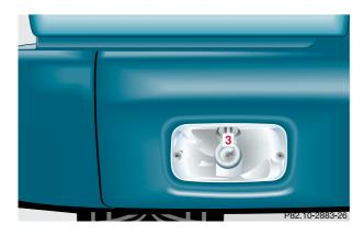
3 Bulb for backup lamp/rear fog lamp P 21W 12V
