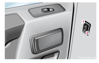
The switch is located on the center pillar.
