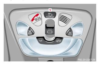
1 Press button (1) to switch the cargo compartment lamps (2) on/off.
