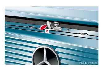
Lift hood up slightly. Pull safety hook (2) in direction of arrow and open hood.
