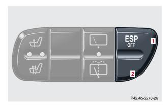
ESP control switch located in center console.
