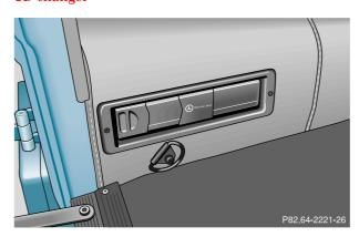
The CD-changer is located in the left side of the cargo compartment.
