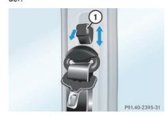
1 Button for belt outlet height adjustment
