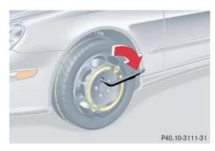
► Unscrew the alignment bolt, install last wheel bolt and tighten slightly.
