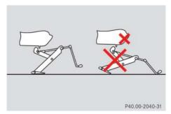
▶ Jack up the vehicle until the wheel is a maximum of 1.2 in (3 cm) from the ground. Never start engine while vehicle is raised.
