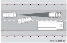
Distronic has not yet detected the vehicle changing lanes. There will be insufficient distance to the lane changing vehicle.
