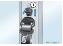
Button for belt outlet height adjustment
