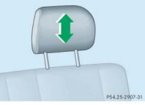
Manually adjust the height of the head restraint.
