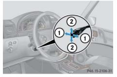
Adjusting steering column, in or out
