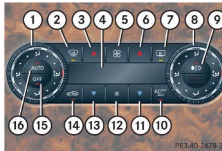
Automatic climate control panel design A
