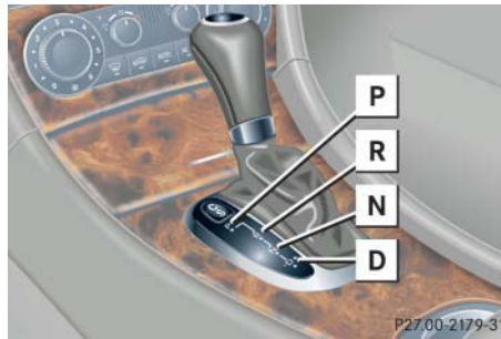
Gearshift pattern for automatic transmission
