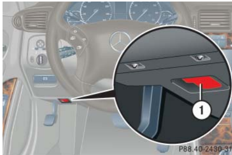
① Hood lock release lever
