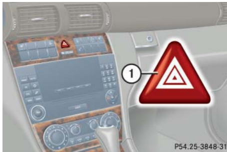
① Hazard warning flasher switch
