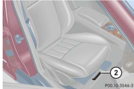
② Vehicle Identification Number (VIN)
