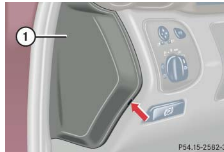
① Main fuse box cover
