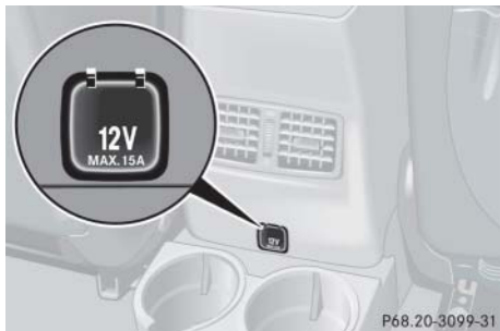
Electrical outlet in the rear passenger footwell
