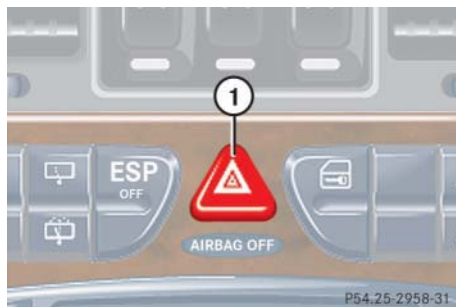
① Hazard warning flasher switch
