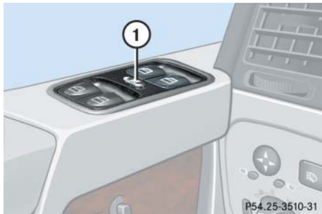
① Override switch
