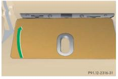
Lift cargo floor plate at rear edge (arrow).
