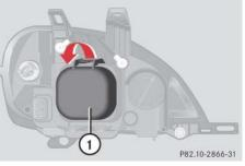
Low beam halogen or Bi-Xenon\* housing cover with locking tab
