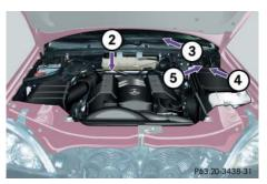
(2) Engine number (engraved on engine)(3) VIN, visible (lower edge of windshield)
