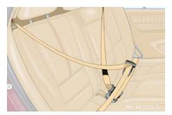
For additional safety when transporting cargo while the rear seats are unoccupied, fasten the outer seat belts crosswise into the opposite side buckles.
