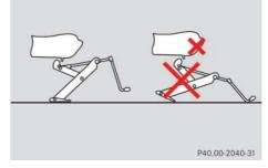
Jack up the vehicle until the wheel is a maximum of 1.2 in (3 cm) from the ground. Never start engine while vehicle is raised.
