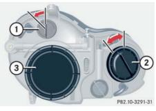
(1) Bulb socket for turn signal lamp
