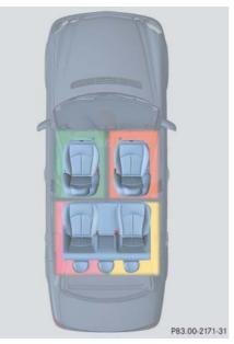
With the help of a sun sensor, the climate control determines the relation of the sun to the vehicle and automatically adjusts the inside temperature for every individual zone.
