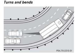
In turns or bends, Distronic may not detect a moving vehicle in front, or it may detect one too soon. This may cause your vehicle to brake late or unexpectedly.
