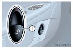
Remote tailgate release switch with indicator lamp
