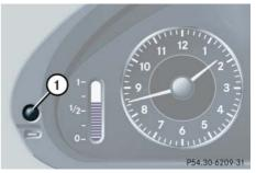
Press the reset button ① on the left side of the instrument cluster.
