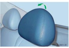
Swing the head restraint forward by hand until it engages.
