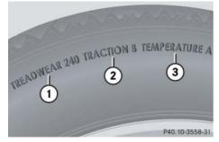
Quality grades can be found, where applicable, on the tire sidewall between tread shoulder and maximum section width. For example:
