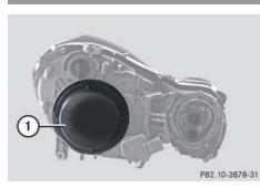
Housing cover for low beam halogen or Bi-Xenon\* headlamp
