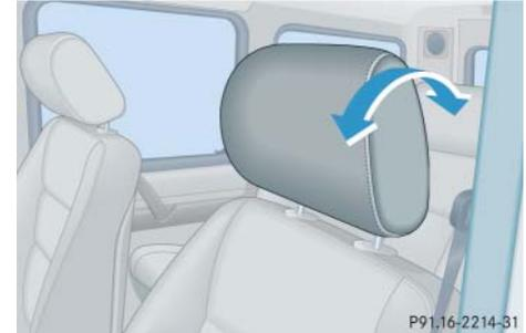
Manually adjust the angle of the head restraint.
