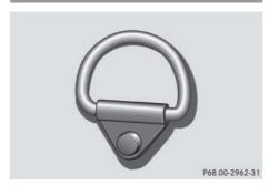
The cargo compartment is provided with four tie-down anchors.
