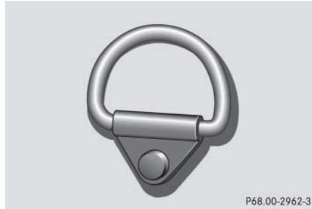
The cargo compartment is provided with four tie-down anchors.
