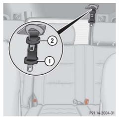
Pull both latch plates ① and ② out of the attachment (▷ page 45).
