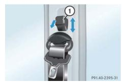
① Button for belt outlet height adjustment
