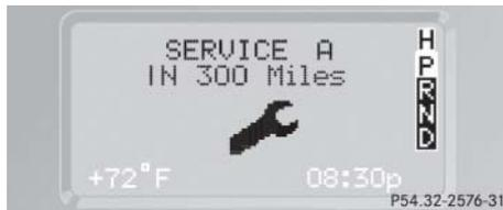
The type of maintenance service due is indicated in the speedometer display field:
