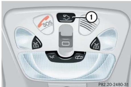
① Switch for cargo compartment lamps
