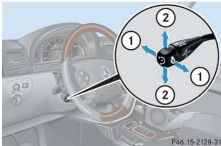
① Adjusting steering column, in or out
