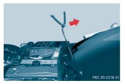
Slide the wiper blade out in direction of arrow.
