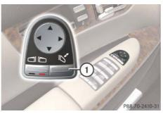
(1) Folds the exterior mirrors in and out
