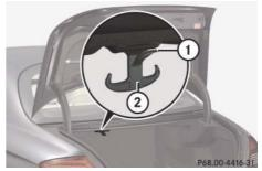
▶ Pull tab ① of retaining hook ② down.
