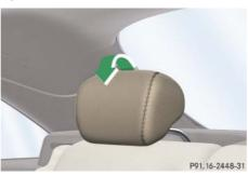
Pull the rear seat head restraint upright until it locks into place.
