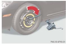
Unscrew the alignment bolt, install the last wheel bolt and tighten slightly.
