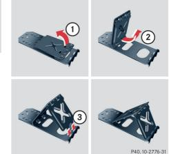
Tilt the plate upward
