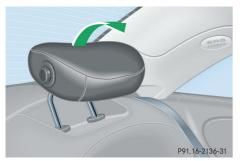
Pull the rear head restraint forward until it locks into position.
