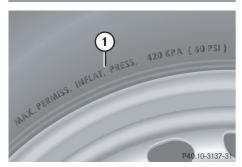
Maximum permissible tire inflation pressure **(**) For illustration purposes only. Actual data on tires are specific to each vehicle and may vary from data shown in above illustration.
