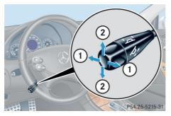
Adjusting steering column, in or out
