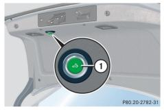
**()** The emergency release button unlocks and opens the trunk while the vehicle is standing still or in motion.
