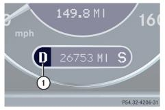
1) Current gear selector lever position
