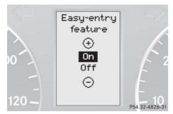
► Press button ← or ← to switch the easy-entry/exit feature 0n or 0ff.
