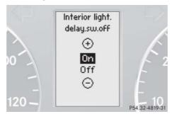
Press button for or to switch the interior lighting delayed shut-off feature 0n or 0ff.
