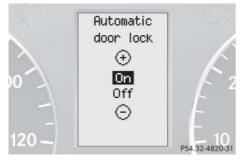
Press button or to switch the automatic central locking 0n or 0ff.
