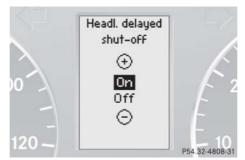
Press button + or to switch the headlamps delayed shut-off feature 0n or 0ff. ► Turn the exterior lamp switch to position AUTO before turning off the engine.
