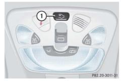
(1) Switch for cargo compartment lamps
