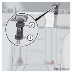
Pull both latch plates ① and ② out of the attachment (▷ page 50).
