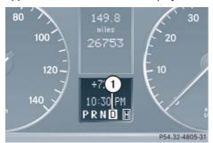
(1) Current gear selector lever position
