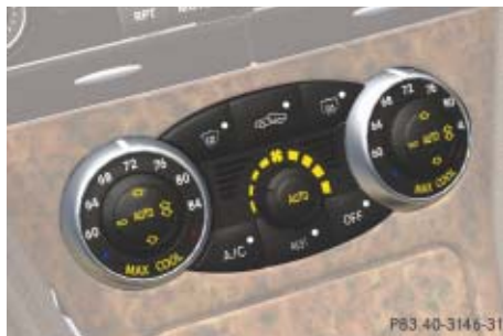
Automatic climate control panel with MAXCOOL activated
