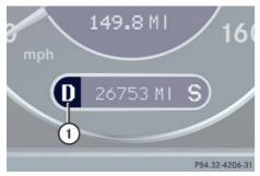
(1) Current gear selector lever position
