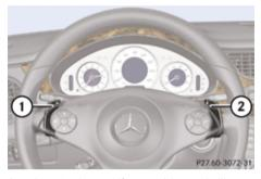
Steering wheel gearshift control (example illustration)
