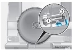
▶ Open lock (1) using the screwdriver.
