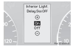
Press button + or - to switch the interior lighting delayed shut-off feature On or Off.
