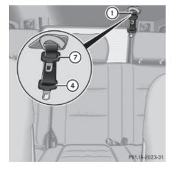
Pull both latch plates ④ and ⑦ out of attachment ①.
