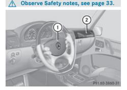
Driver's front air bag ① and front passenger front air bag ② are designed to provide increased protection for the driver and front passenger against the risk of injuries to the head and thorax.
