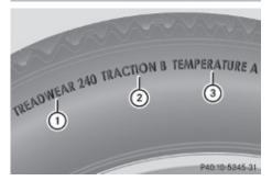
The Uniform Tire Quality Grading is a U.S. Government requirement designed to give drivers consistent and reliable information regarding tire performance. Tire manufacturers are required to grade tires based on three performance factors: treadwear ①, traction ②, and temperature resistance ③. Although not a Government of Canada requirement, all tires made for sale in North America have these grades branded on the sidewall.
