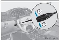
Press the combination switch in direction of arrow (1) or (2).
