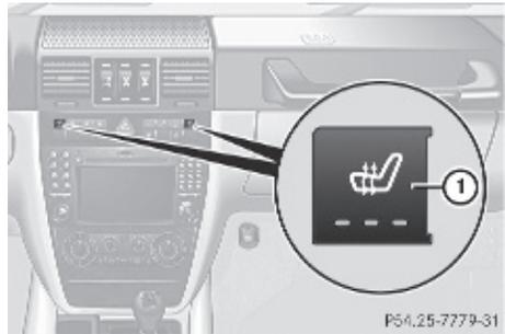
The red indicator lamps in the switch come on to show which heating level you have selected.
