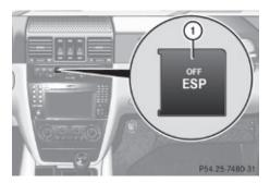
▶ With the engine running, press ESP<sup>®</sup> switch ① until the ESP<sup>®</sup> warning lamp
