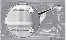
The brake fluid level is correct when it is between lower mark (MIN) ② and upper mark (MAX) ① of the brake fluid reservoir.
