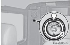
The warning indicator is divided into four yellow and two red distance segments (1). The Rear Parking Assist system is ready to measure when you hear a signal and readiness indicator (2) is illuminated.
