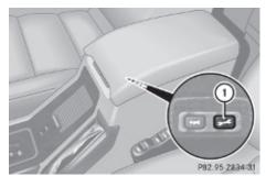
Press and hold Roadside Assistance button ① for longer than 2 seconds. A call to a Mercedes-Benz Roadside Assistance dispatcher will be initiated. The indicator lamp in Roadside Assistance button ① will flash while the call is in progress. The message Connecting Call will appear in the multifunction display and the COMAND system is muted.
