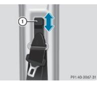
Raising: Slide the seat belt outlet height adjuster upward.
