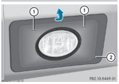
Example illustration: Right front fog lamp (left front fog lamp laterally reversed)
