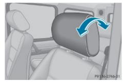
Adjust the head restraint to the desired position by pushing or pulling on the upper edge of the head restraint cushion.
