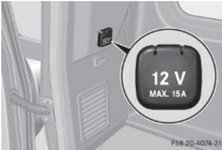
If the engine is off and the power outlets are being used extensively, the vehicle battery may become discharged.
