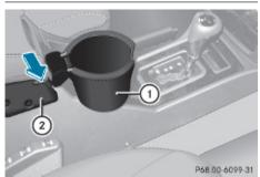
Place bracket of cup holder (1) into recess indicated by arrow of cup holder base (2).
