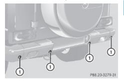
To function properly, sensors ① must be free of dirt, ice, snow and slush. Clean sensors ① regularly, being careful not to scratch or damage sensors ①, see "Cleaning the Rear Parking Assist system sensors" (▷ page 190).
