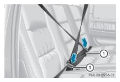
For additional safety when transporting cargo while the rear seats are unoccupied, fasten the outer seat belts crosswise into the opposite side buckles (1).
