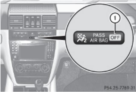
Special BabySmart™ compatible child seats, designed for use with the Mercedes-Benz system, are required for use with the BabySmart™ air bag deactivation system. Please contact an authorized Mercedes-Benz Center for information on availability. With the special child seat installed properly, the front passenger front air bag will not deploy.
