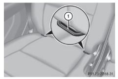
LATCH-type anchors ① are located between the seat cushion and the backrest.
