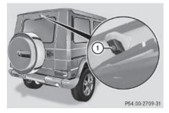
Camera lens ① must be free of dirt, ice, snow, and slush to function properly. Clean the camera lens regularly. Being careful not to scratch or damage the camera lens, see "Cleaning the rear view camera lens" (▷ page 190).
