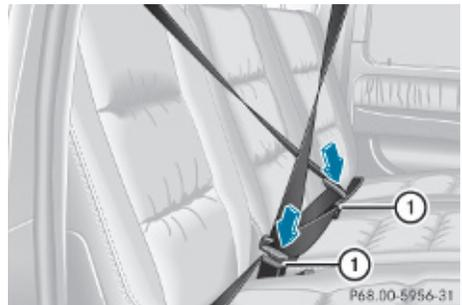
For additional safety when transporting cargo while the rear seats are unoccupied, fasten the outer seat belts crosswise into the opposite side buckles ①.
