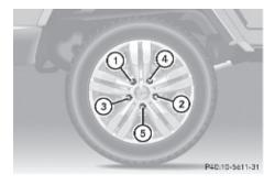
Tighten the five wheel bolts evenly, following the diagonal sequence illustrated (1 to 5), until all bolts are tight. Observe a tightening torque of 96 lb-ft (130 Nm).
