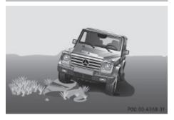
Obstacles can damage the vehicle underbody or suspension components. If possible use the assistance of a second person outside the vehicle to scout the path you intend to take and check for adequate ground clearance when you cross obstacles with your vehicle. The person assisting you outside the vehicle should always be a safe distance away from the vehicle and positioned so that he or she cannot get hurt in case of any unexpected vehicle movement.
