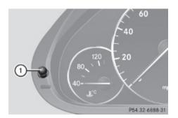
Clearing the maintenance service indicator message manually: Press reset button ① on the instrument cluster. The standard display appears in the multifunction display.
