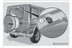
Only use clean water and a soft, nonscratching cloth to clean rear view camera lens (1).
