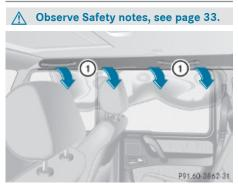
When deployed, window curtain air bags ① are designed to provide increased protection for the head (but not the chest or arms) of the occupants on the side of the vehicle on which the impact occurs.
