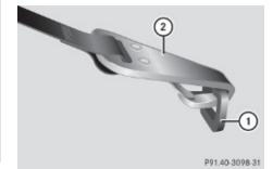
For safety, make sure hook ② is attached to anchorage ring ① beyond the safety catch, as illustrated.
