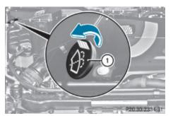
Fluid for the washer system, rear window washer system, and the headlamp cleaning system is supplied from the washer fluid reservoir.
