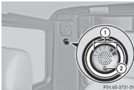
The warning indicator is divided into four yellow and two red distance segments ①. The Rear Parking Assist system is ready to measure when you hear a signal and readiness indicator ② is illuminated.
