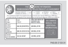
The Tire and Loading Information placard lists the recommended cold tire inflation pressures ① for maximum loaded vehicle weight. The tire inflation pressures listed apply to the tires installed as original equipment.
