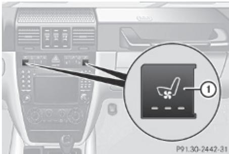
The blue indicator lamps in seat ventilation switch ① come on to show which ventilation level you have selected.
