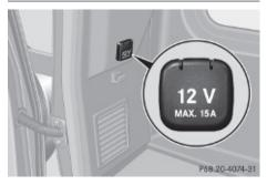
If the engine is off and the power outlets are being used extensively, the vehicle battery may become discharged.
