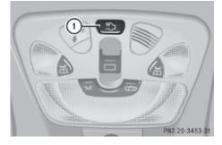
Switching rear interior lamp on/off: Press switch ①.
