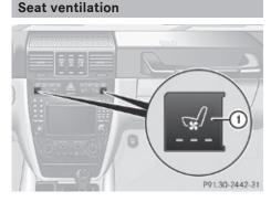
The blue indicator lamps in seat ventilation switch 1 come on to show which ventilation level you have selected.
